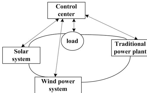
Fig. 1. Typical structure of VPP
